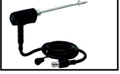
Industrial probe for interchangeable probe tubes with 9' or 16' sampling line and heated probe handle and easy replaceable quartz glass wool filter Available with and without heated sampling line
